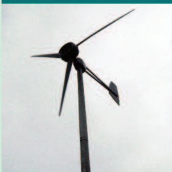
5Kw wind turbine
